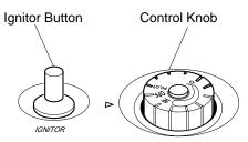
Figure 15 - Control Knob In The OFF Position
